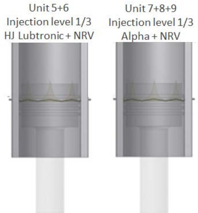
Figure 8: Setup of unit 5+6 & unit 7+8+9
