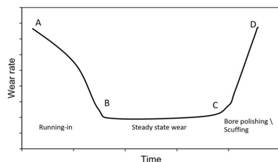
**Figure 1:** Normal wear profile for lubricated systems.
