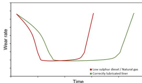
**Figure 2:** Correctly lubricated liner increases the steady state wear and prevent early bore polishing and scuffing.
