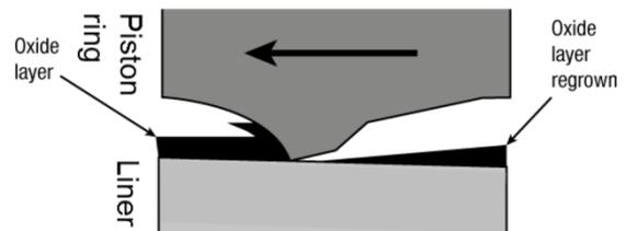
Figure 3 Schematic representation of oxide layer removal – exposing the surface to corrosion
