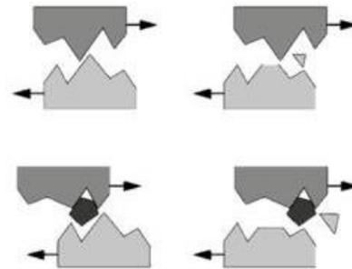
Figure 2 Schematic representation of abrasive wear
