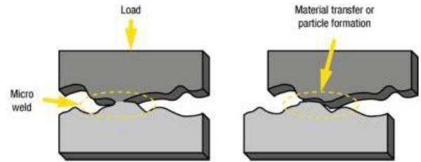
Figure 1 Schematic Representation of Adhesive Wear
