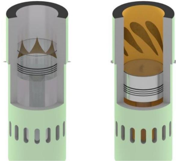
Figure 5: Left: Ring Pack Lubrication, Right: HJ SIP Lubrication
