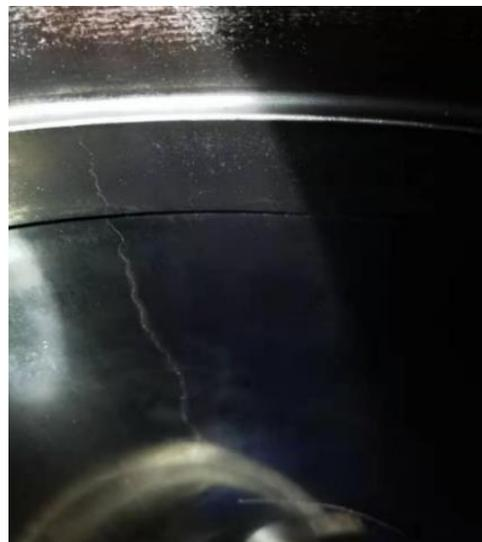
**Figure 1.** Cracked cylinder liner.
