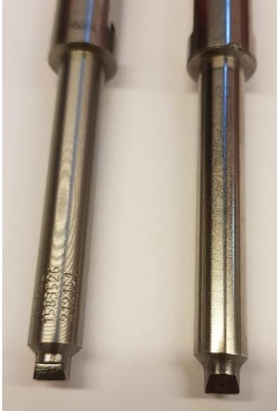
**Figure 2.** Counterfeit nozzle might not have serial numbering.
