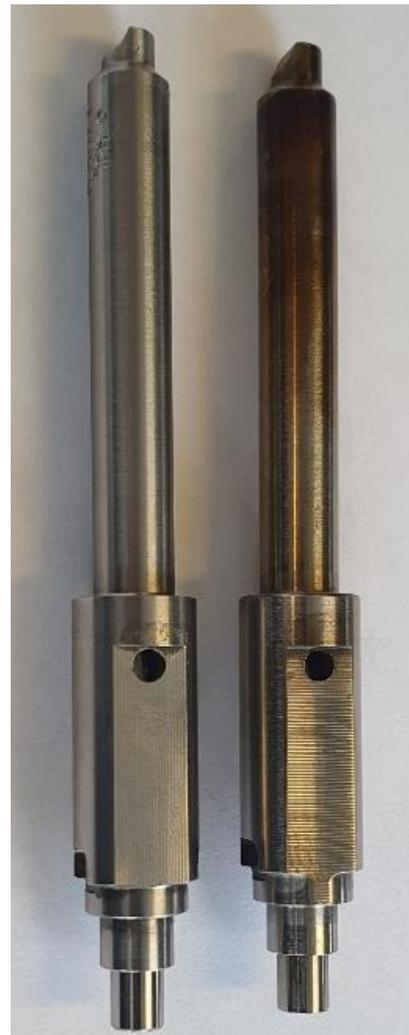
Above photo shows 2 nozzles for the HJL SIP valve. The right is a non-genuine nozzle and the left one is a genuine HJL nozzle. All new original HJL nozzles are clearly marked and can easily be identified.
