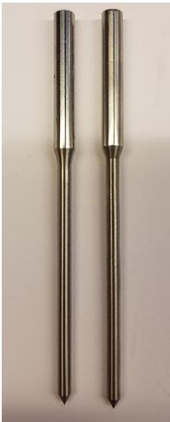
**Figure 3.** An OEM needle and a counterfeit need.
