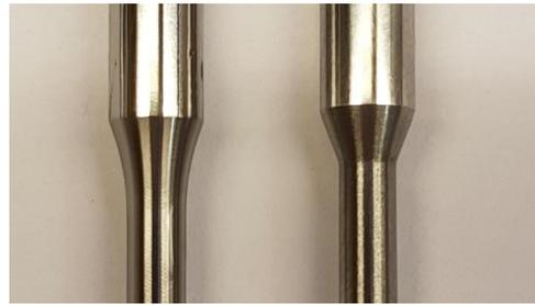
**Figure 3.** Close-up of identification point. The original nozzle will have a soft reduction in diameter of the nozzle.
