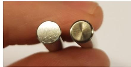
**Figure 4.** Close-up of identification point. The original nozzle will have a sharp transition from the sides to the top.
